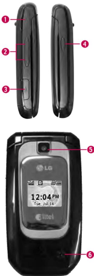
1. **Earphone Jack** Allows the use of a headset for handsfree conversations.
